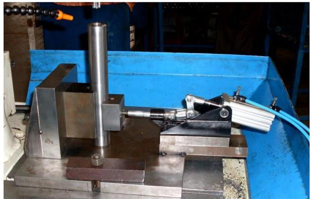
AOT-2530-HTC used to hold cylindrical w/p in tapping process
