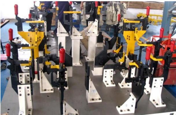
Numerous HV Series used in a Spot welding fixture
