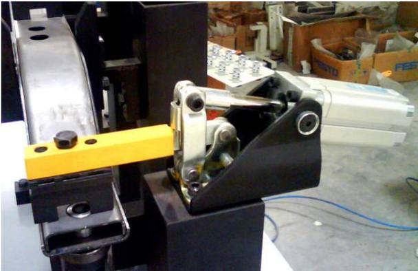
AOT-3586-SB used in a checking fixture
